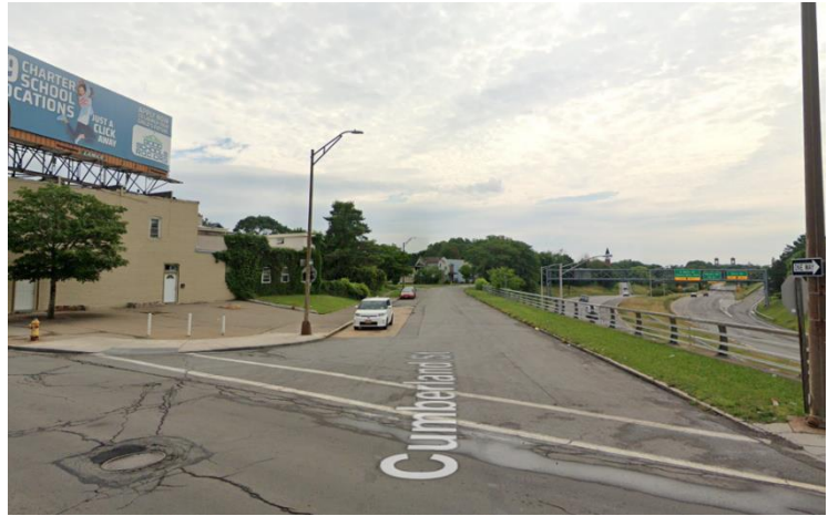
A narrow, one-sided sidewalk and long crossing distance at Cumberland Street, an Inner Loop parallel service road.
